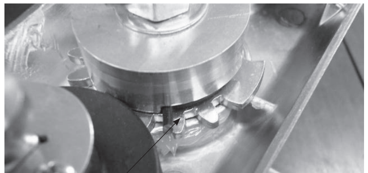
Spring orientation for right hand reverse operation
