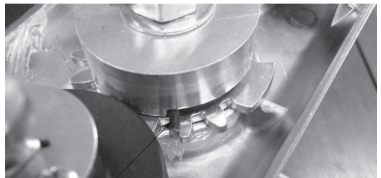
Spring orientation for right hand reverse operation
