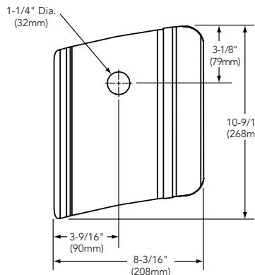
Designed for exterior doors that require extra security or resistance to vandalism, anti-vandal trim (AVT) plates have an extended lip on the active side of the door to provide extra protection for the latchbolt. A matte plastic coated grip provides a comfortable pull over wide temperature ranges. Fully through-bolted with no exposed exterior fasteners for a cleaner look and increased security.
