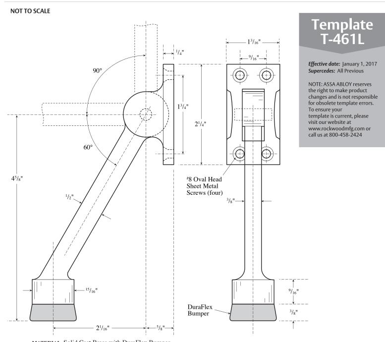
MATERIAL: Solid Cast Brass with DuraFlex Bumper
