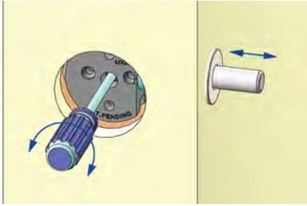
4.4) Ensure spindle hub is at center of trim bore. Use spindle or screwdriver to test bolt retraction; if not smooth, troubleshoot as follows:
