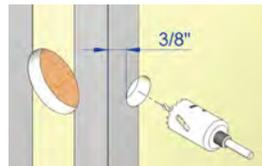
3.2) For dry wall or flat casing openings, use a 1" hole saw to cut lock bore hole to depth as shown in chart.
