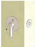
5.3) Fasten trim screws until trim is tight to jamb surface. NOTE: Do not over tighten.
