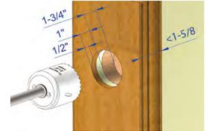
**NOTE:** In Step 2.3, if there is a gap between the drywall and the stud, measure the distance and add to the bore hole depth. Hole depth must accommodate lock barrel preparation in Step 4. You can deepen trim bore as needed after that step.
