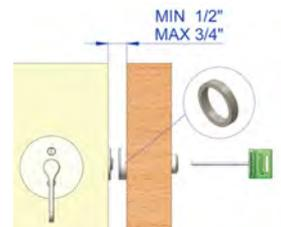
6.4) Install the 1" dust-proof strike with the 1/4" release screws on the outside.
