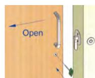
6.7) Use release key (provided with lock set) to push through center hole on release to push lock bolt back and unlock door.
