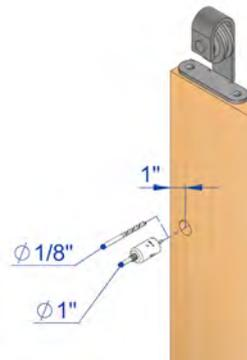
6.3) With the pilot hole as a guide, use a 1/4" bit to drill a hole from the outside to connect with the strike bore hole.
