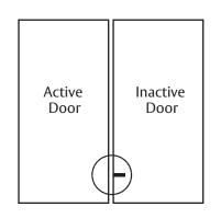
IMPORTANT: The 19BFB will project during a fire. Do not cover with any edge mounted door hardware.
